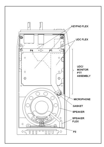
Figure 9 - Speaker, Microphone And Flex Circuit Access
